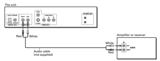
• Connect the unit's AUDIO OUT to any line-level inputs (such as AUX, DVD, CD, etc.) of an audio amplifier or receiver.
